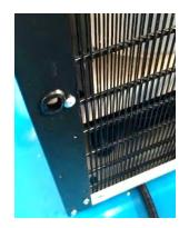
Fit the rubber grommet into the hole that has either been drilled for mini models or knocked out for free standing models. The grommet is used to protect the harness as it goes through the machine.
