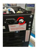
**For Free Standing models only:** Carefully knock through the knockout hole for the pedal wire harness to go through. It may be necessary to enlarge the knockout hole using a 17mm drill bit for the grommet to fit appropriately.
