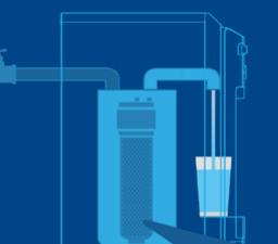
Waterlogic filters adsorb particles and contaminants without filtering minerals essential to your wellbeing
