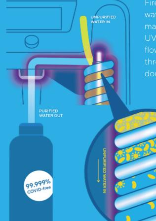
Firewall exposes water from the mains supply to UVC radiation as it flows down then up through the unique double-helix spiral
